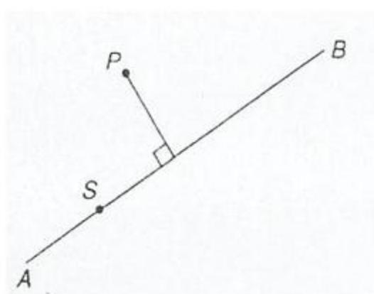
In the diagram above, the ship S (or plane) is travelling on a straight line AB. The shortest distance to point P is when SP is perpendicular to AB.
